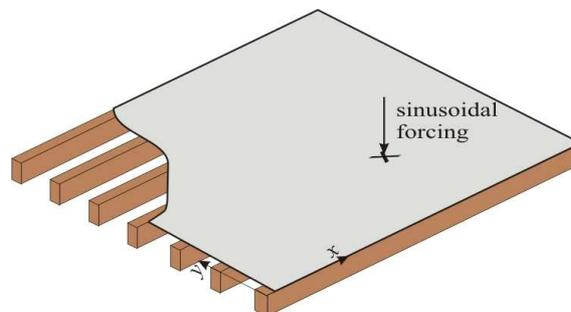
Figure 1: Drawing depicting the design of a joist floor. The structure has equally spaced joists running parallel to each other. The origin of the coordinate system is placed at the corner of the structure.
