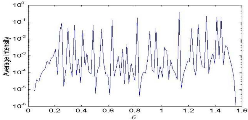
Figure 2: Average intensity in a rectangular plate, 7m by 3.2m, Young's modulus 14GPa, Poisson ratio 0.3, mass density per unit area 620 Kg
